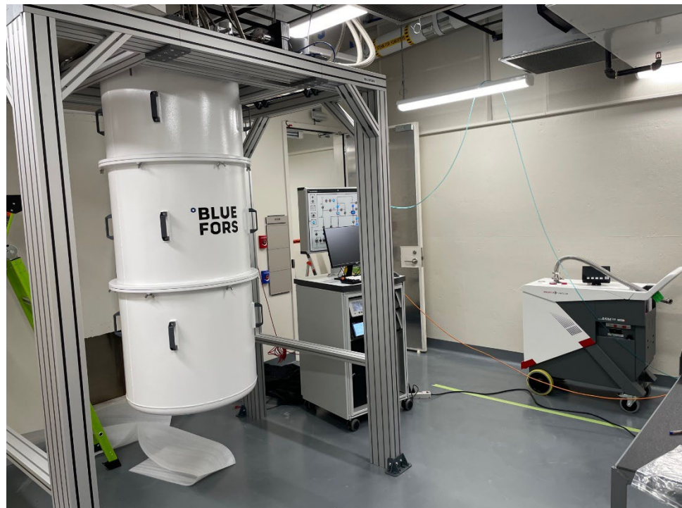
Figure 4: A dilution refrigerator, which creates the ideal environment for qubit performance, at Argonne Quantum Foundry
